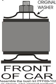
Assemble the bush kit PFF69-102 as shown. Use original washers. Reverse only the washer which is nearest the locating nut.
